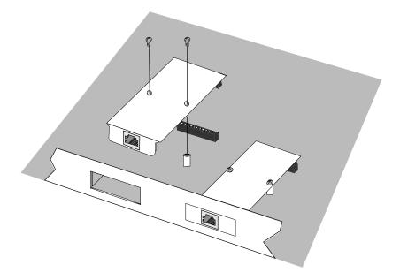
Figure 3-1. Installing an FPIM
